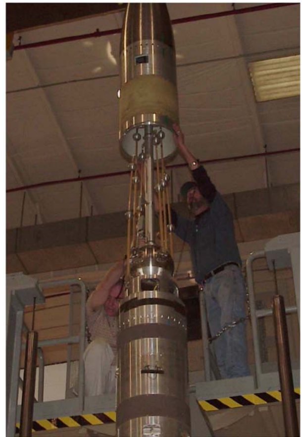
FIGURE 5 | Electric field probes as deployed in sounding rocket 21.116.
