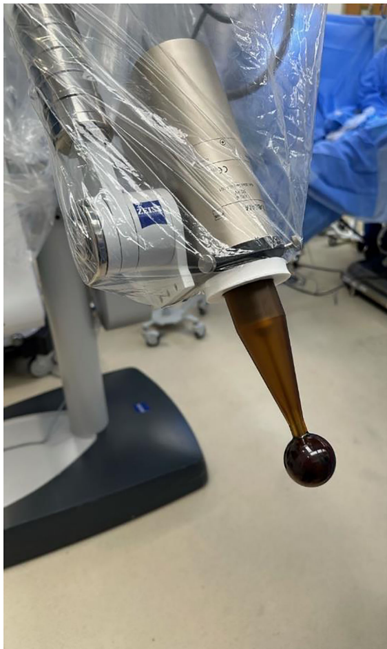
FIGURE 1 Dressed IntraBeam 600 miniaturized 50 kV X-Ray linear accelerator with 40 mm applicator mounted (Zeiss, Oberkochen, Germany).
