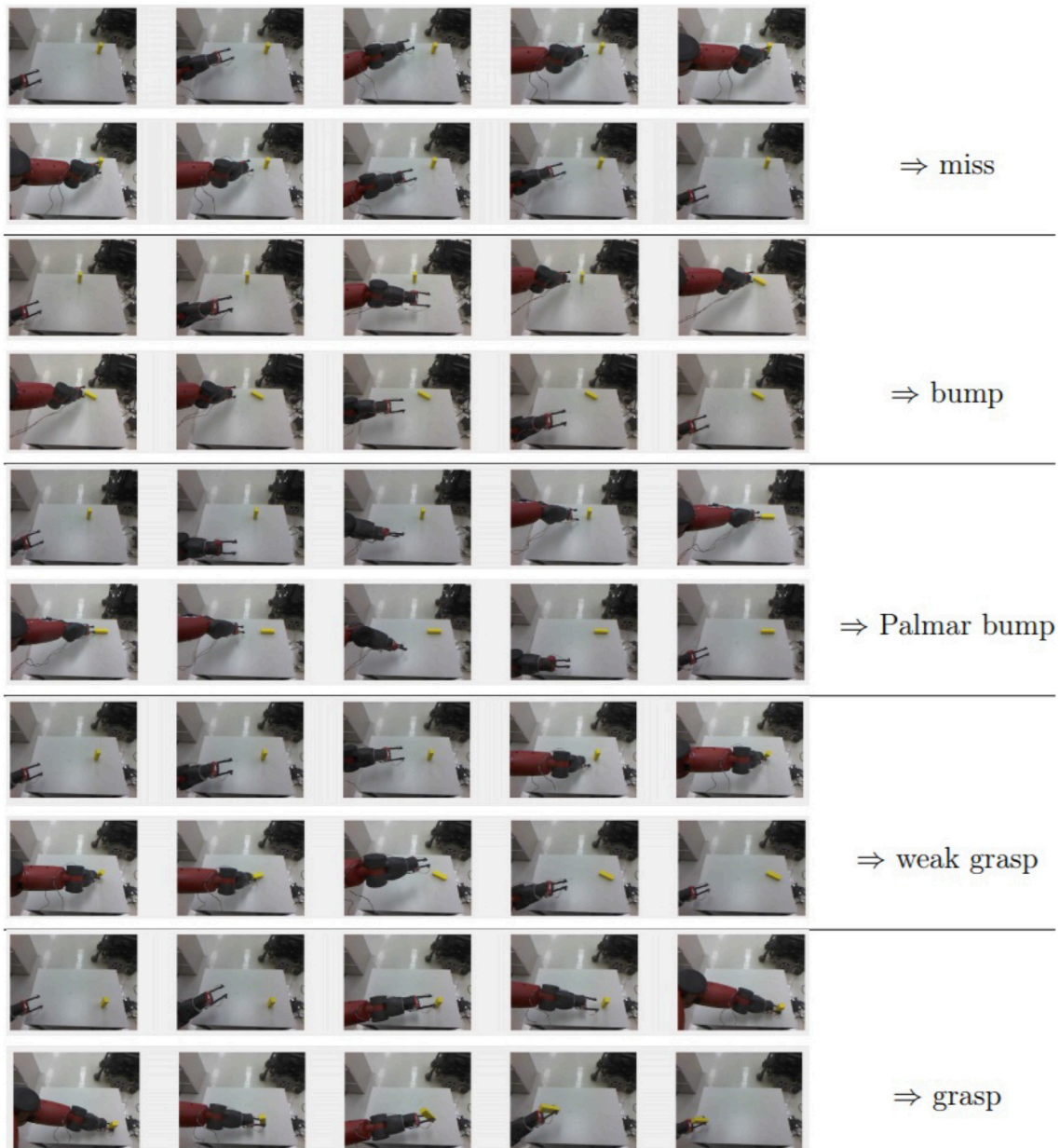
FIGURE 8 | The agent's RGB percepts during attempted grasp trajectories. Images for the forward portion toward n_f are shown in the first of each pair of rows, and images for the portion to return to n_h are shown in the second rows. Images for some nodes in the middle of trajectories with more than five nodes have been omitted. The agent classifies the result of the grasp attempt by observing the state of the target object during the trajectory. In all cases but miss , there is a substantial change between the first and last observations, and the trajectory is a successful reach. In all other cases these observations should be significantly different, and the reach component of the grasp was successful. Further classification depends on the state throughout the return trajectory and if the Palmar reflex was activated, as discussed in section 5.1.1. Only the result of the final example is considered to be a successful grasp.
