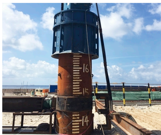
FIGURE 7 High-strain hammer test on pile foundations.
