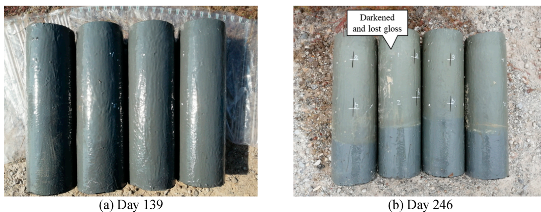
FIGURE 9 Surface morphology changes of LC polyurea anti-corrosion coating. (a) Day 139. (b) Day 246.
