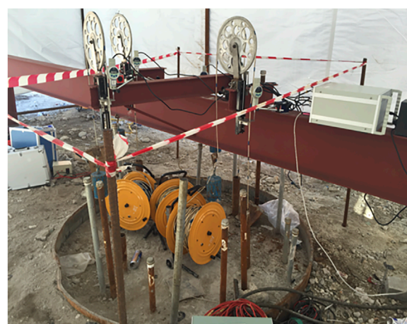
FIGURE 11 Field self-balancing pile test.
