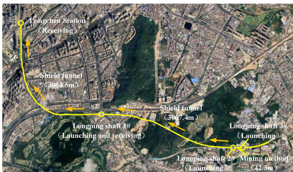
FIGURE 2 Schematic plan of the route in Work Zone 1 for the Dapeng Branch Line of the Shenzhen-Huizhou Intercity Railway.
