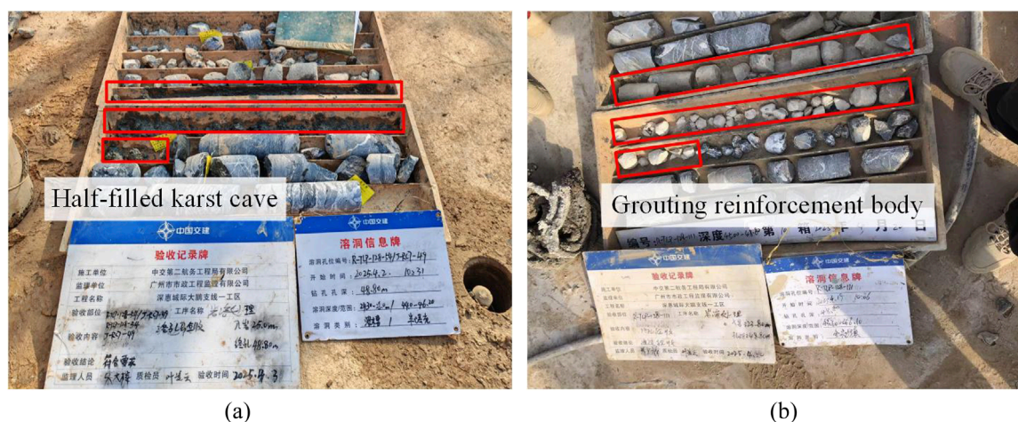
FIGURE 12 Comparison of rock cores before and after grouting. (a) Before grouting. (b) After grouting.
