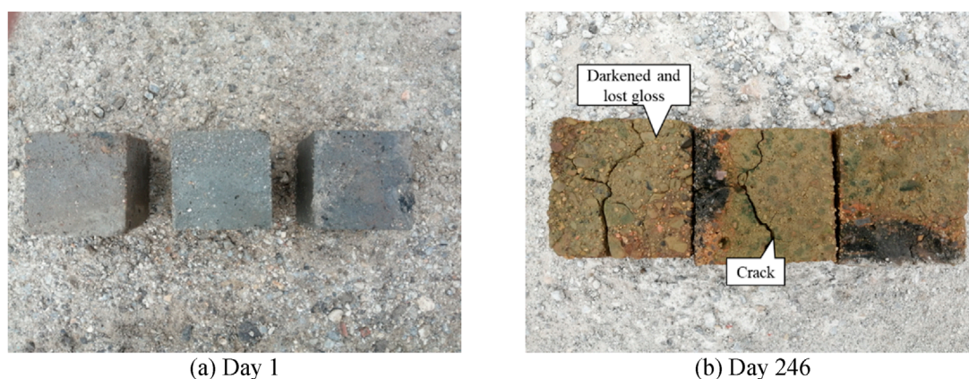
FIGURE 10 Surface morphology changes of uncoated concrete. (a) Day 1. (b) Day 246.
