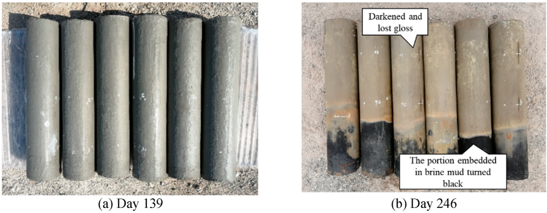
FIGURE 7 Surface morphology changes of ZH acrylic anti-corrosion coating. (a) Day 139. (b) Day 246.
