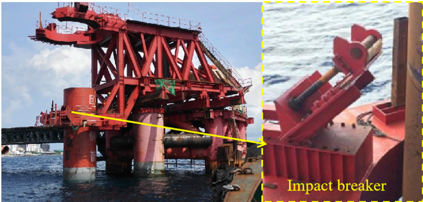
FIGURE 12 Guide frame with hydraulic automatic opening and closing chuck and impact breaker.
