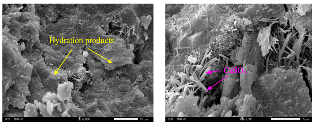
FIGURE 14 Micro-morphology of CGSs for 120d under karst water erosion.
