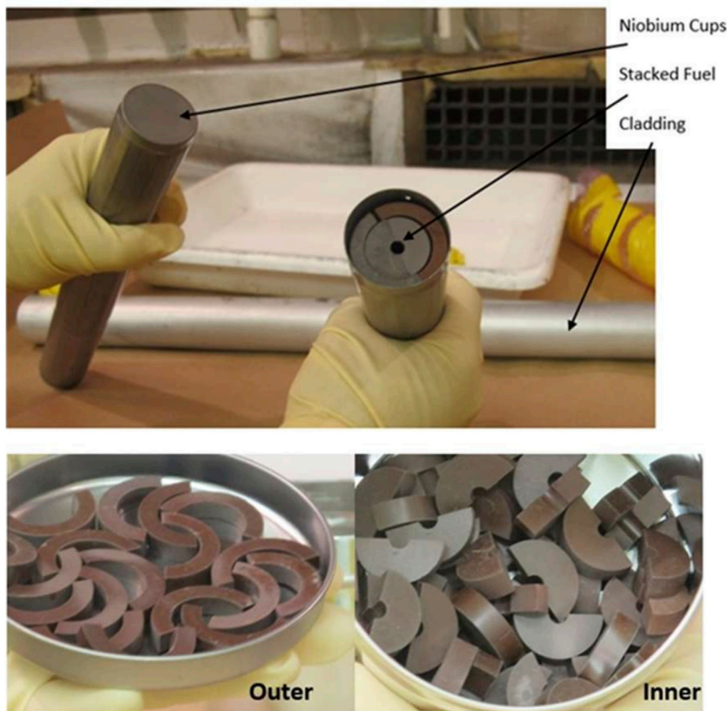
FIGURE 3 Photograph of fuel and niobium cups showing inner and outer fuel disks (Ames et al., 2022).
