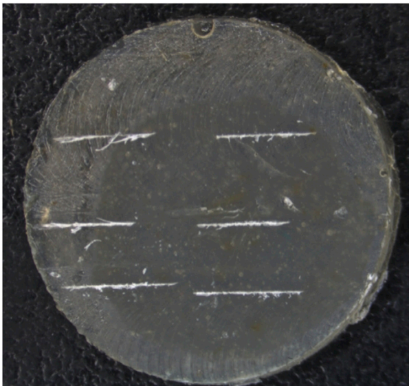
FIGURE 2 The resin disc samples with six artificial scratches.
