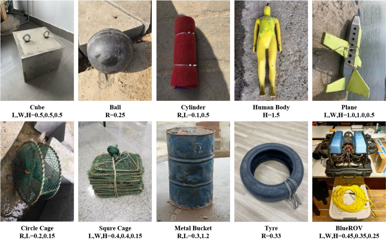
FIGURE 8 The physical sonar target entities and their corresponding size in the UATD dataset. The size is measured in meters.
