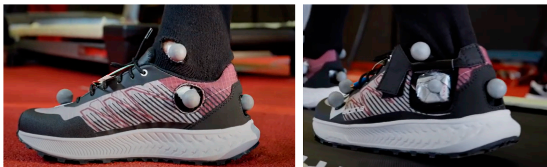
FIGURE 3 Adapted running shoes with modifications for attaching markers, with openings under the medial malleoli and the heel.
