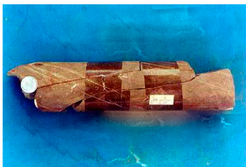
FIGURE 3 Characteristics of core fractures of Jurassic Ahe Formation in the Dibe area.
