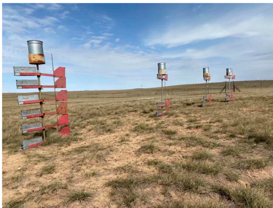
FIGURE 2 BSNE dust sampler field photo.
