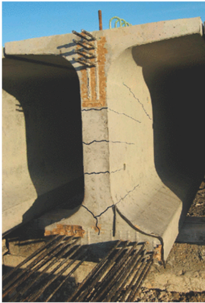
FIGURE 1 End zone cracks in a precast prestressed concrete beam (derived from Okumus and Oliva, 2013).
