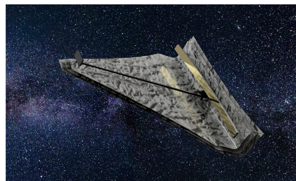
FIGURE 1 Concept design for a rectangular space telescope, modeled after DICER and JWST. The primary mirror is made of twenty 1\text{ m} \times 1\text{ m} beryllium mirror segments. Scaling from JWST, the secondary mirror is 1\text{ m} \times 2.3\text{ m} and deployed about 23 m away and offset from the primary mirror. The sunshield is meant to allow observations in all sky directions, though mirror position angles will be limited in directions that are at large angles from the antisolar point. During launch, two 10 m sections of mirrors can be folded with the reflective sides together, next to the secondary mirror support and a folded sunshade. After the two mirrors unfold, the secondary mirror beam extends out, dragging the triangular portion of the sunshade with it. The folded payload could reasonably fit in a space that is 11\text{ m} \times 2.5\text{ m} \times 2.5\text{ m} , plausibly fitting in a Falcon Heavy launch vehicle.
