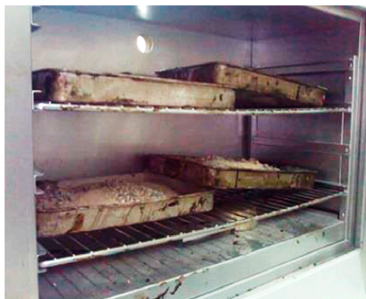
FIGURE 4 Pre-heating of (A) aggregate in oven, (B) bitumen in oven.
