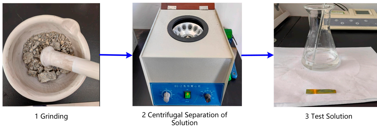
FIGURE 4 Preparation of test solution.
