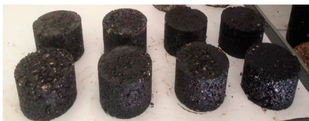
FIGURE 3 Bituminous samples prepared using the Marshall mix design method.
