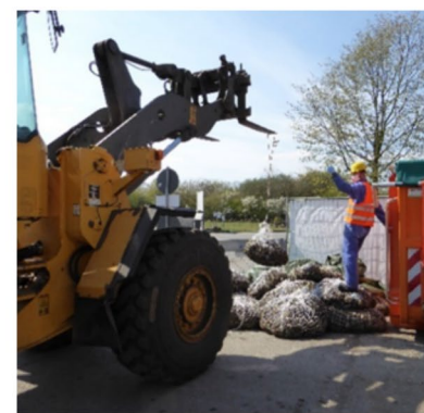
Determination of net mass with a crane scale
