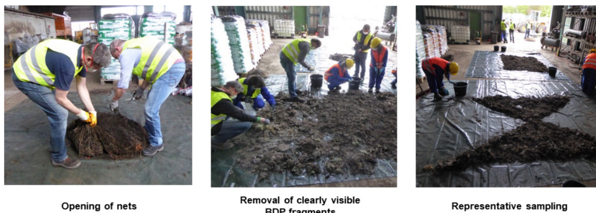
FIGURE 6 Preparation of samples for further analytics (partially based on Deegener et al., 2022).
