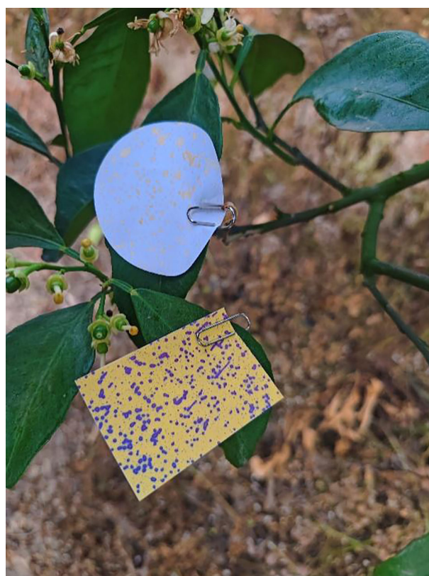
FIGURE 7 The water-sensitive paper and filter paper after the spray test.
