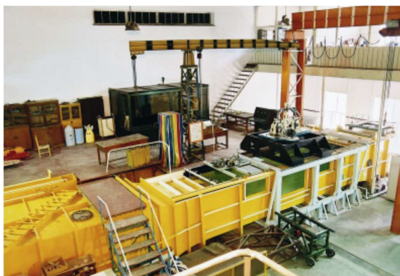
FIGURE 2 Circulating water channel used for the experiment.
