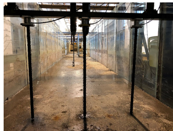
FIGURE 5 Local physical model test with scale of 1:20.
