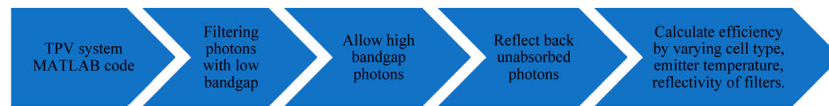
FIGURE 4 | Flow chart representing the followed methodology which represents the mentioned procedure in the form of a flow chart which explains the TPV system is modeled using MATLAB which encounter the variables that stops the low bandgap photons reaching the front surface of TPV cell then BSR variables reflects the unabsorbed photons back to the front side of the TPV cell.
