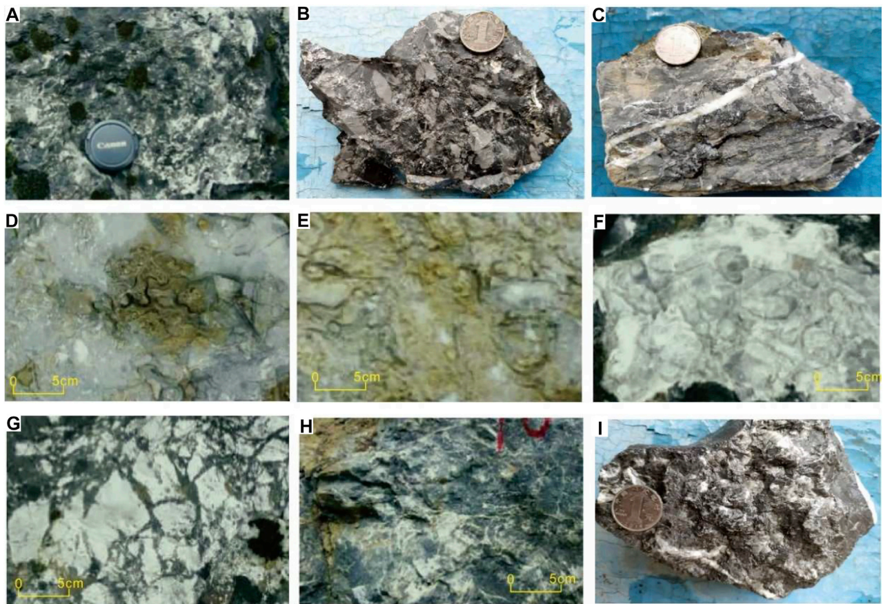
FIGURE 4 | Lithology and biology of Changxing Formation reef in outcrop of Jiantianba. (A,B) Algal reef limestone, mainly composed of blue-green algae, content up to 65%; (C,D) algal bonded sponge reef limestone, with about 25% sponge content and 35% blue-green algae content, has obvious algal bonded—barrier structure; (E) sponge skeleton reef limestone, with obvious barrier—skeleton structure, reef-building organisms are mainly string sponges and fiber sponges, the content of which is about 60%; (F) skeleton reef limestone, with biological skeleton structure, reef-building organisms are mainly string sponges, fiber sponges, etc.; (G) limestone breccia, breccia for angular, for the collapse of the reef formation; (H,I) light grey blocky dolomitic reef limestone, fracture and dissolution of the geode is developed well.
