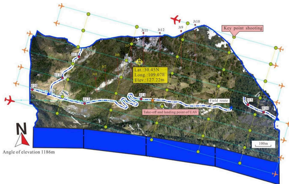
FIGURE 8 | 3D digital outcrop model processed by UAV oblique photography, outcrop of Jiantianba. The maximum resolution of a local image was ~10–20 cm. Cruise line automatic set-up by POS system. The UAV take off from start point to the end then achieved outcrop scanning and taking pictures.
