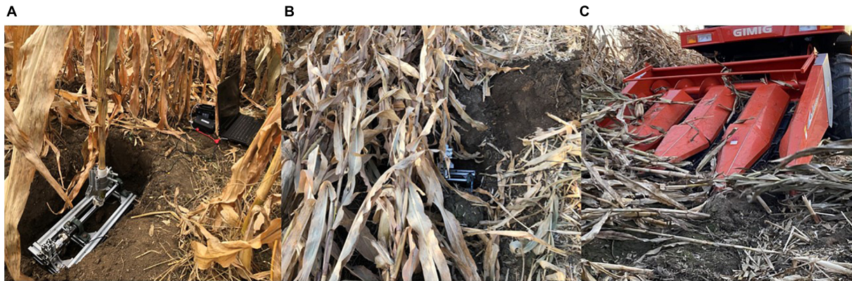
FIGURE 3 | An experiment of forces on stalks in corn harvesting. (A) Experiment on the upright corn; (B) experiment on the lodged corn; (C) the experiment scene of corn harvest.
