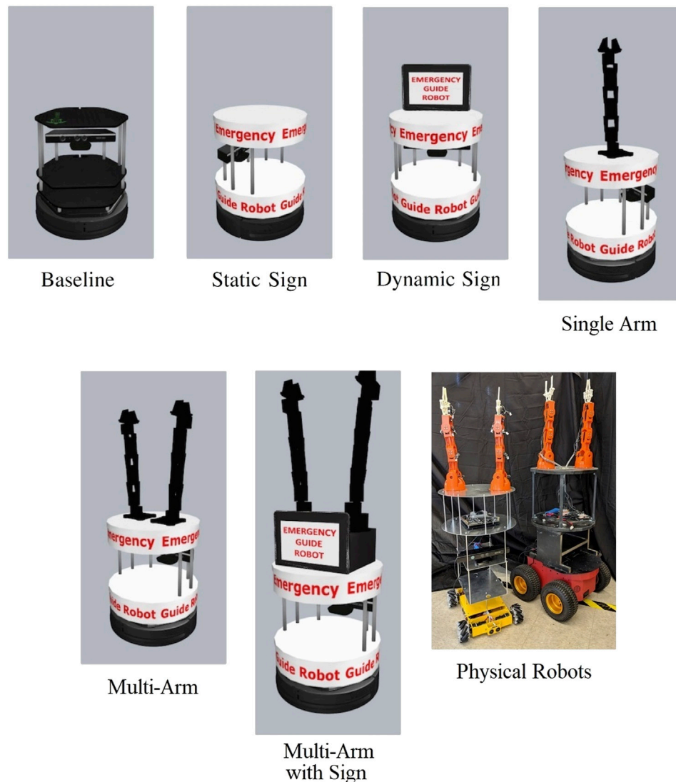
FIGURE 6 | Different robot designs evaluated for its ability to communicate guidance directions. The physical robots are based on the multi-arm design.
