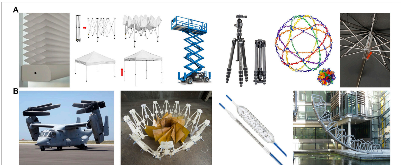
FIGURE 1 | Expandable structures are found in a variety of everyday items, such as window shades, canopies, construction equipment, tripods and stands, toys, and umbrellas (A). Expandable structures are also used in a variety of industrial and scientific purposes, including foldable aircraft, satellite design, medical devices, and architecture (B).
