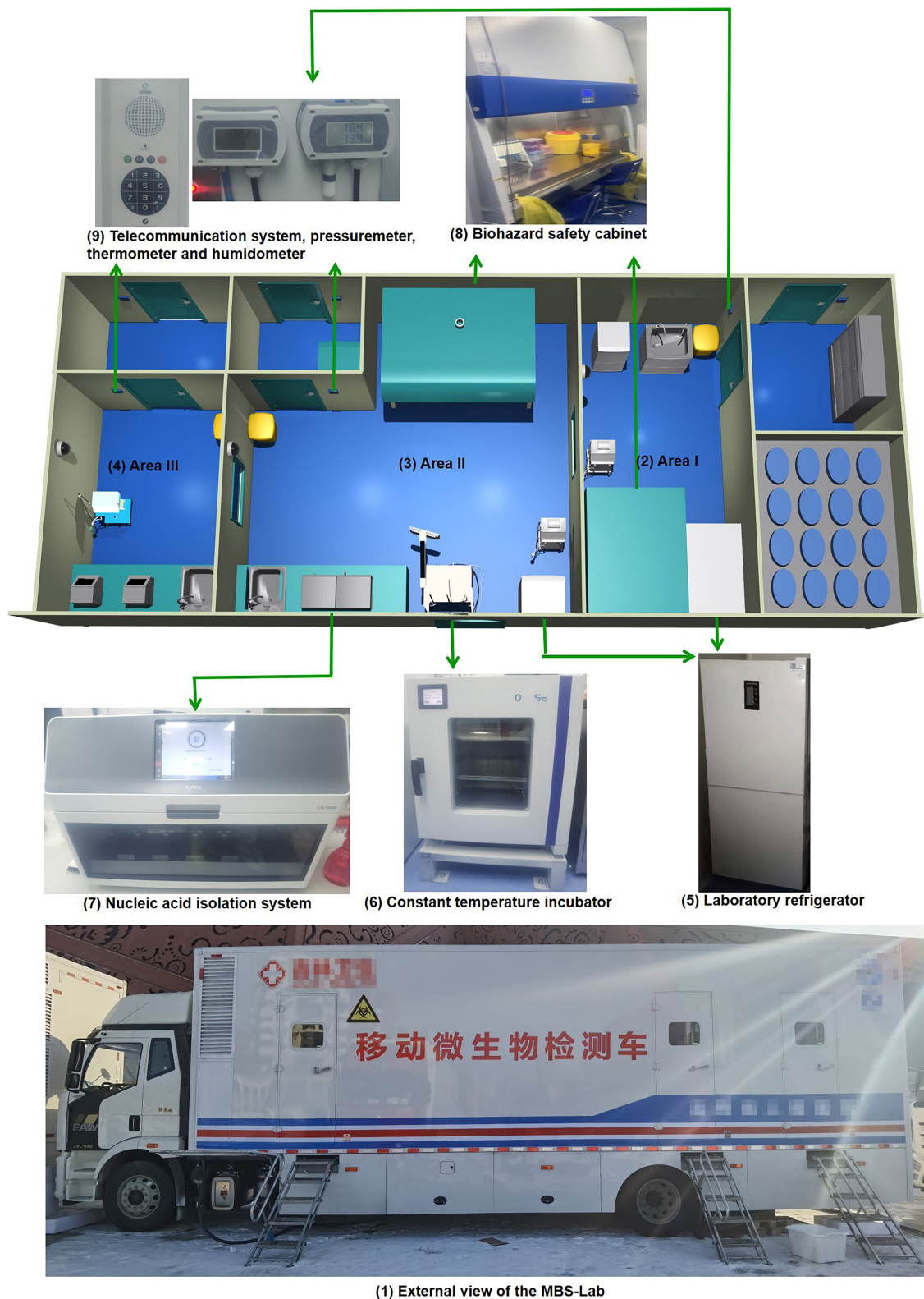
FIGURE 1 | Layout of main devices in the mobile biosafety laboratory. (1) External view; (2) area I; (3) area II; (4) area III; (5) laboratory refrigerator; (6) constant-temperature incubator; (7) nucleic acid-isolation system; (8) biohazard safety equipment; (9) telecommunication system, pressure meter, thermometer and hygrometer.
