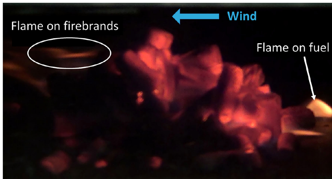
FIGURE 8 | Photograph showing flames present both over the pile of firebrands, downwind and attached to the glowing firebrands, and over the fuel surface, upwind and anchored to the fuel surface.
