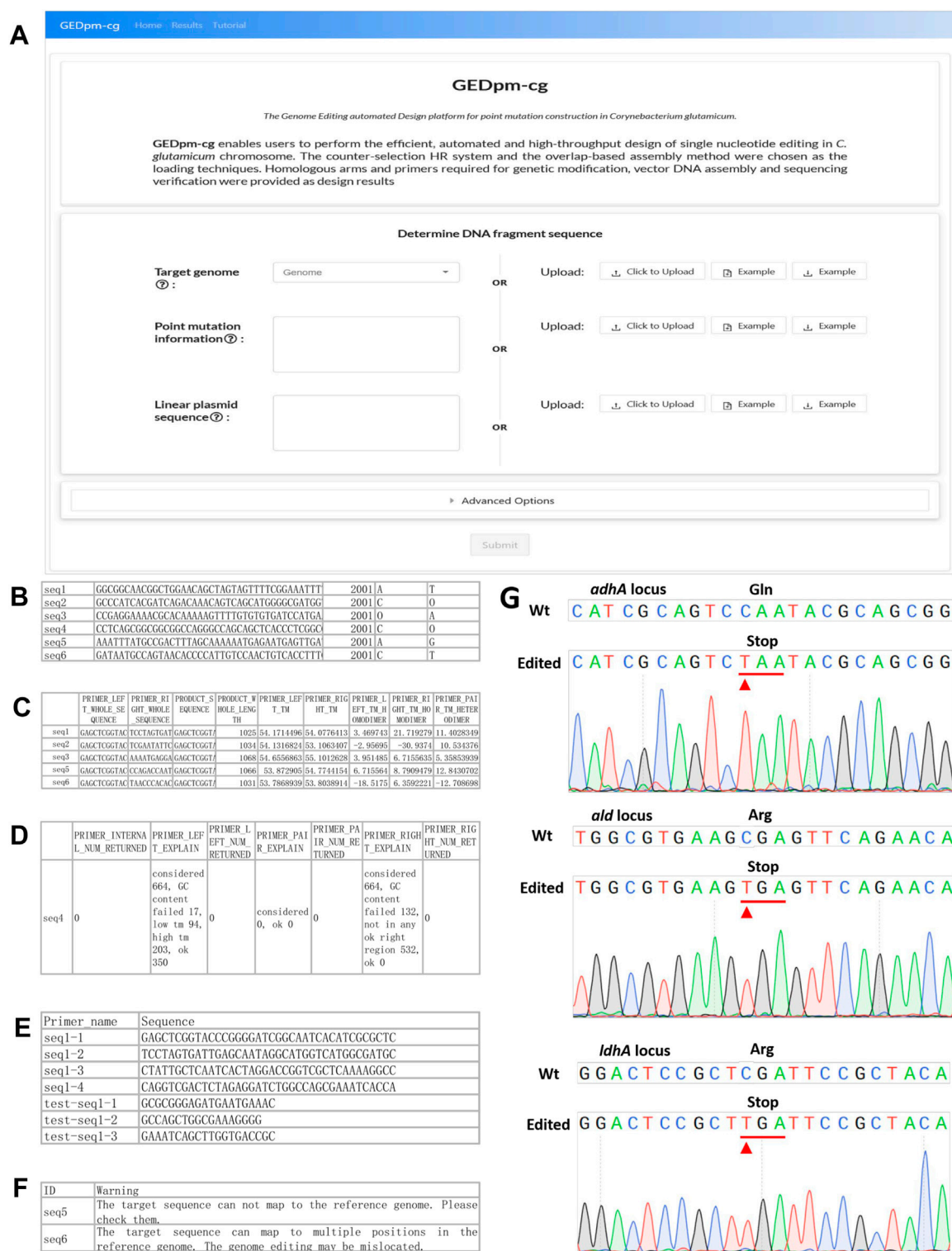
FIGURE 4 | GEDpm-cg web-based interface and examples for input, output and experimental verification. (A) GEDpm-cg web-based interface. (B) Example parts list CSV input file for targeted sequences. (C) Example primer-1 and primer-2, list in XLSX output file. (D) Example primers submitted to the sequence synthesis company, list in XLSX output file. (E) Example of failed primer designs for UHA, list in XLSX output file. (F) Example of possible mis-matching sequences, list in XLSX output file. (G) Sanger sequencing results of point mutation genome editing for adhA C568T , ald C973T and ldhA C463T . The substituted bases are marked with red arrows.
