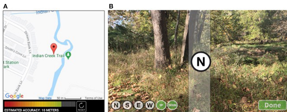
FIGURE 1 | Screenshot of the location accuracy interface (A) and the photo collection tool (B) in the GLOBE Observer app. These tools integrate the phone's functions (GPS, compass, and gyroscope) to ensure land cover photographs are collected uniformly.
