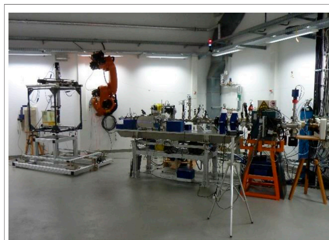
FIGURE 5 | Photograph of the setup. Water phantom inside the frame of the 3D positioning system in front of the accelerator beam line.
