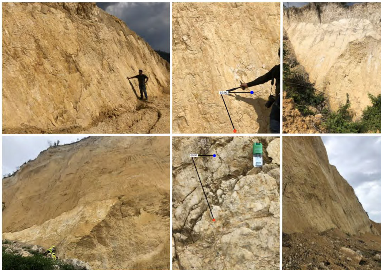
FIGURE 9 | A N66°E fault plane at the landslide head showing slickensides and slickenlines with a 69.9° rake angle. Oblique slip movement is suggested by the direction and orientation of the slickensides.
