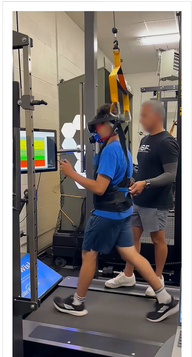
FIGURE 1 Experimental setup during VR walking trials. Participants wore a VR headset and K5 respirometry mask. To mitigate risk of injury, each participant wore a safety harness during all walking trials.
