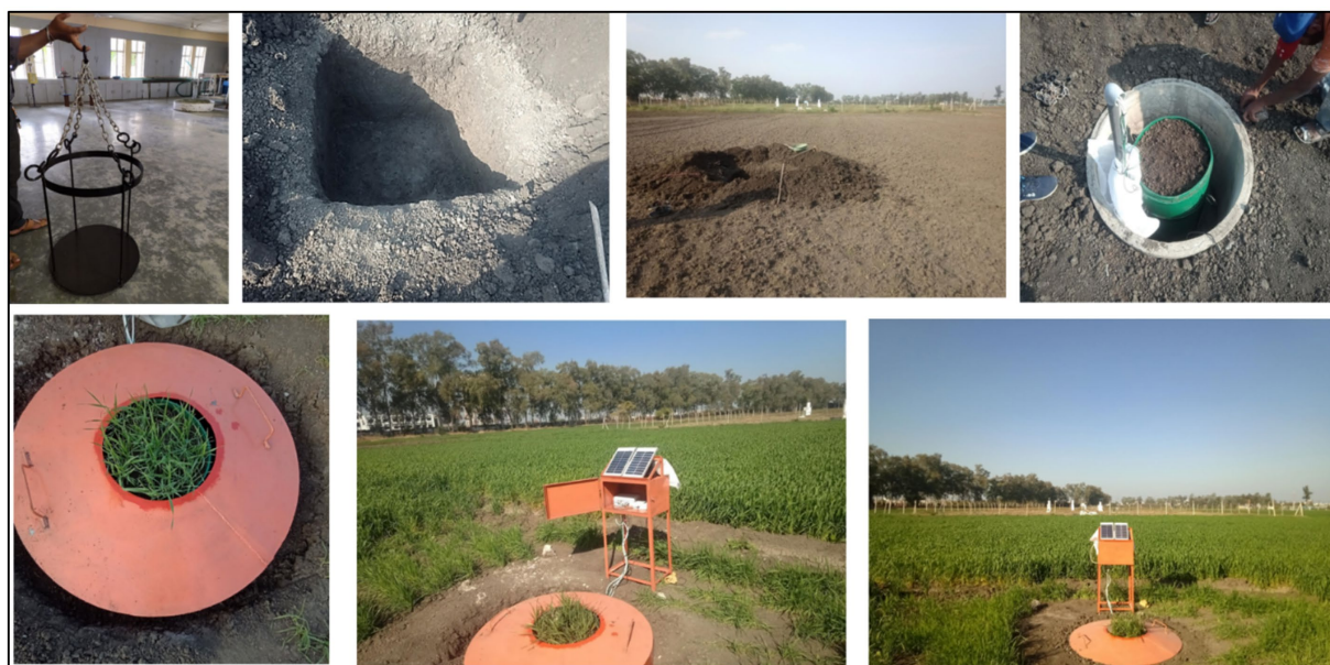
FIGURE 6 Installation of lysimeter in the field.
