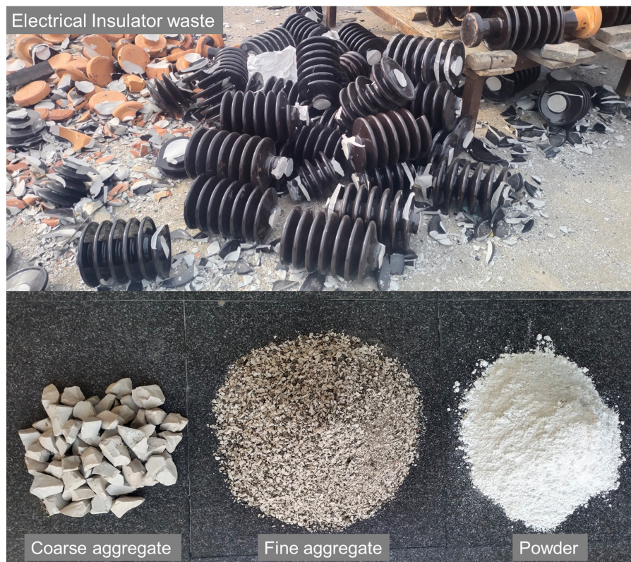
FIGURE 3 Insulator waste as a raw material for concrete.
