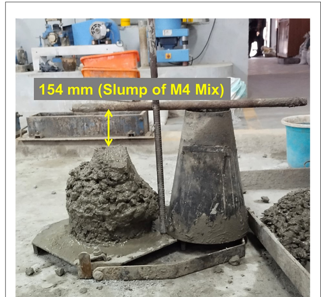
FIGURE 6 Slump test setup.
