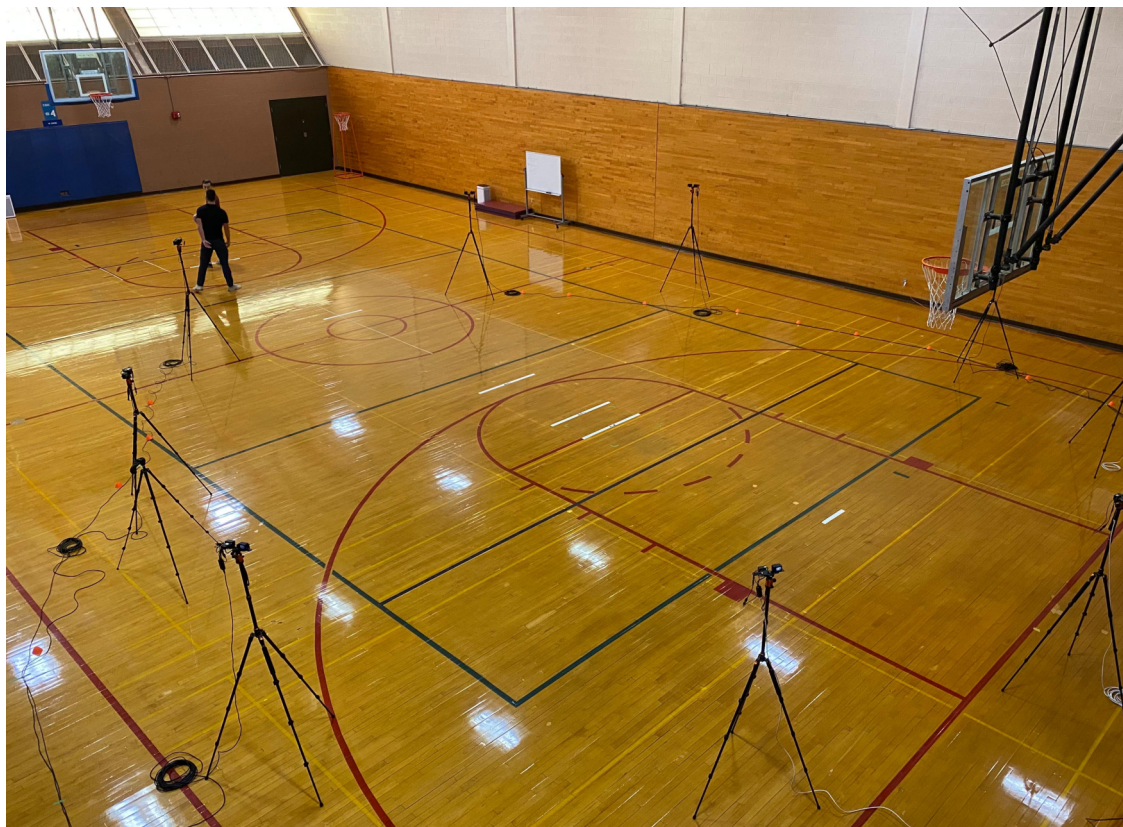
FIGURE 1 A photo of the testing setup, including a markerless motion capture system.
