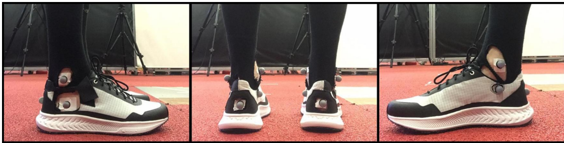
FIGURE 1 Modified Alpina Madeira running shoes featuring openings on the sides and heel to accommodate placement of motion capture markers directly on the skin.
