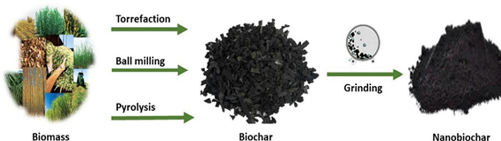
FIGURE 1 The process of fabricating nanobiochar from biochar.
