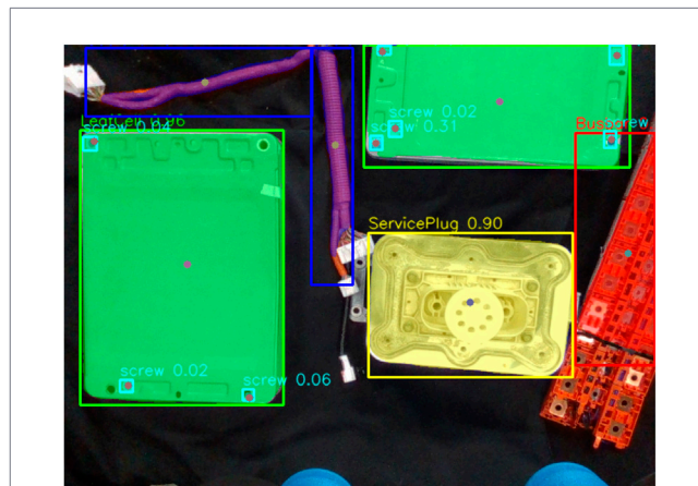
FIGURE 2 Example perception output used by the LLM-ensemble planner. A YOLOv8 model overlays class labels and confidence scores for the battery components (Leafcell, Cable, Busbar, Service Plug, and Screw).
