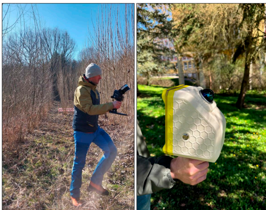
FIGURE 4 Scanning in the plantation - MLS on the left, and a detail of the low-cost MLS prototype is on the right.
