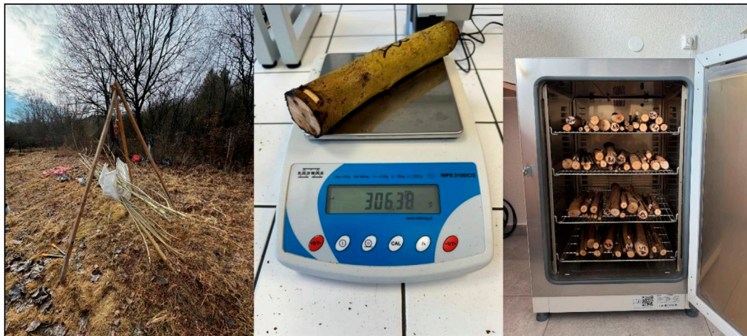
FIGURE 5 Harvesting of research plots: Weighing of the harvested plot in the field (left), weighing of samples in the laboratory (middle), and drying of samples (right).
