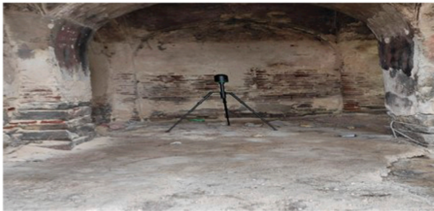
FIGURE 3 Data collection using Leica BLK360.
