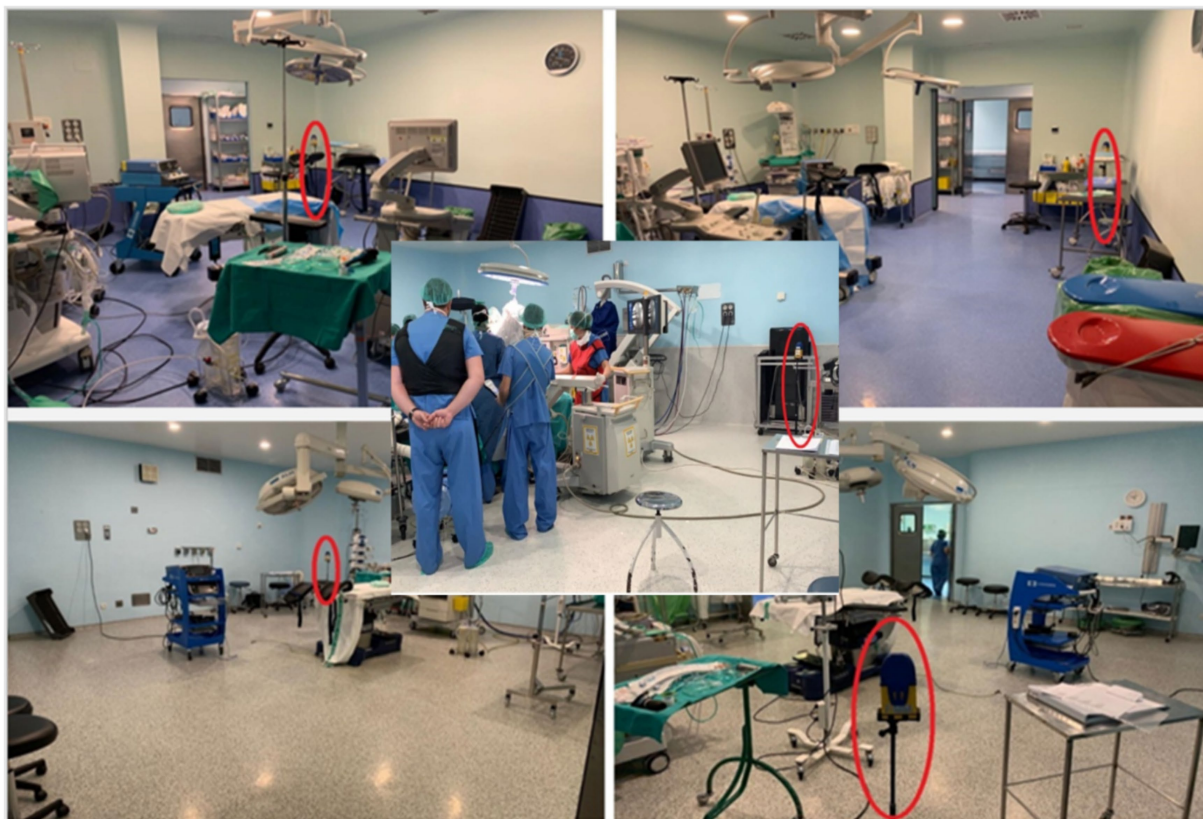
FIGURE 2 Location of the personal exposimeter on a plastic tripod in different operating rooms and situations.
