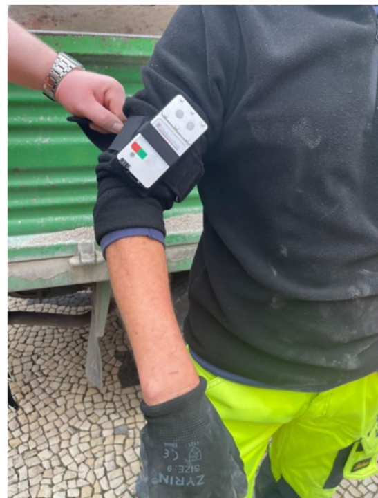
FIGURE 3 Outdoor workers using the GENESIS-UV data logger dosimeter.
