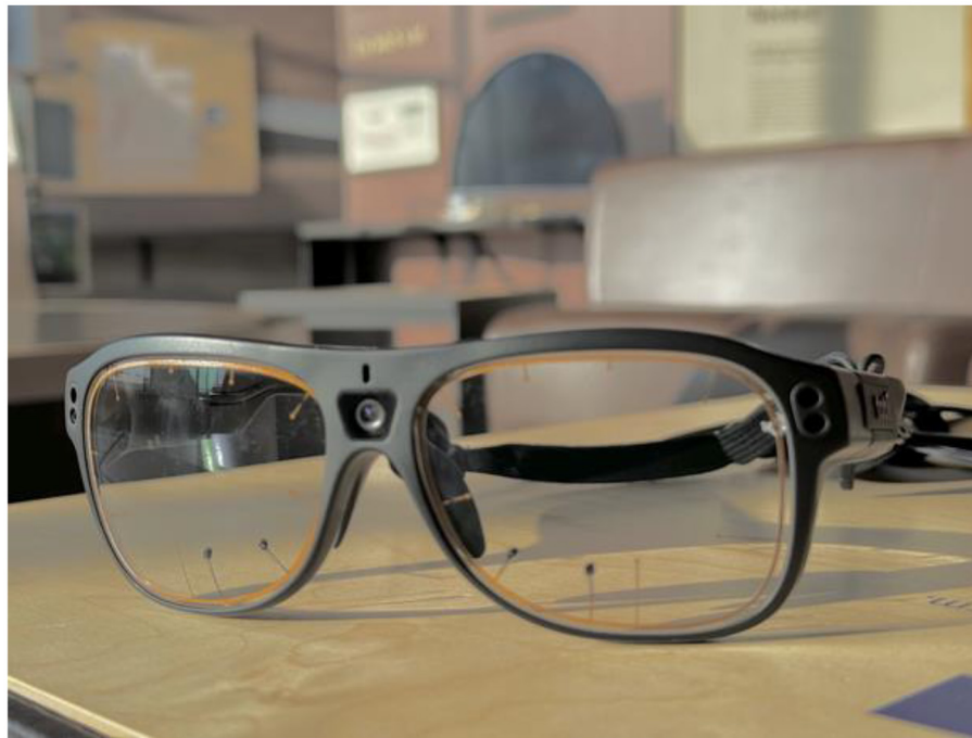
FIGURE 2 Example of a mobile eye-tracker (Tobii Pro Glasses 3) with its illuminators and cameras.
