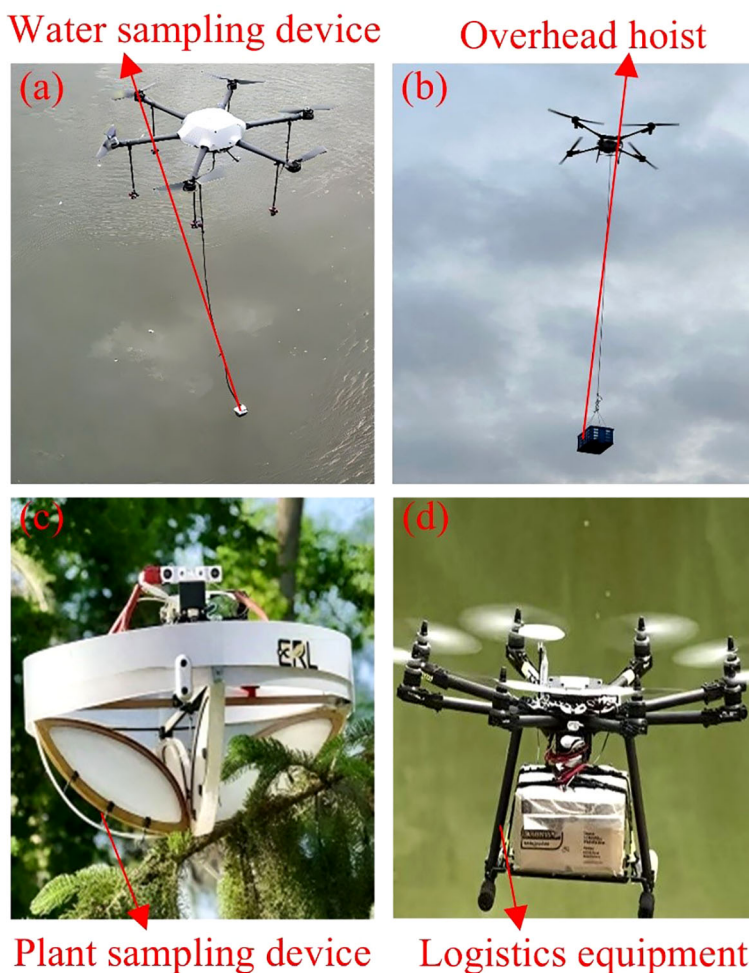
FIGURE 8 UAV-mounted payload interaction devices. (a) UAV equipped with a water sampling device, (b) UAV equipped with a hoisting device, (c) UAV equipped with a plant sampling device, (d) UAV equipped with a logistics transport device.
