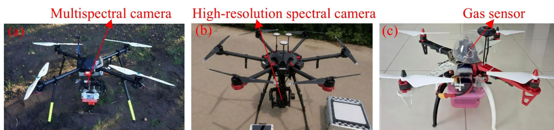
FIGURE 6 Mission-executing sensor types. (a) Multispectral camera mounted on a UAV (Gallego et al., 2018), (b) Hyperspectral camera mounted on a UAV (Liu et al., 2021), (c) Gas sensor mounted on a UAV (Handayani and Suparta, 2022).
