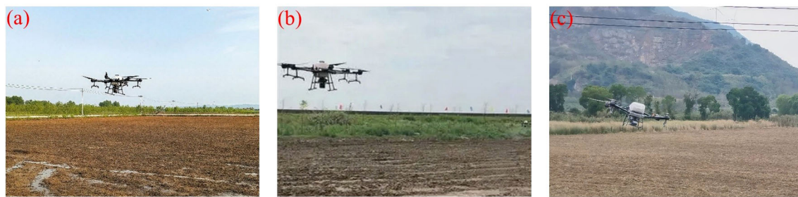
FIGURE 11 Applications of UAV in seeding. (a) Seawater rice seeding, (b) Rice seeding, (c) Wheat capsule seeding.
