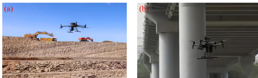
FIGURE 18 UAV applications in engineering surveying. (a) Mining area surveying, (b) Bridge inspection.
