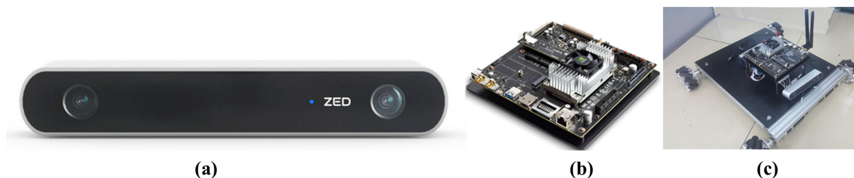
FIGURE 3 Hardware facilities for image acquisition and processing. (a) ZED binocular vision camera. (b) Jetson TX2 edge computing module. (c) McNam wheel omnidirectional mobile platform.
