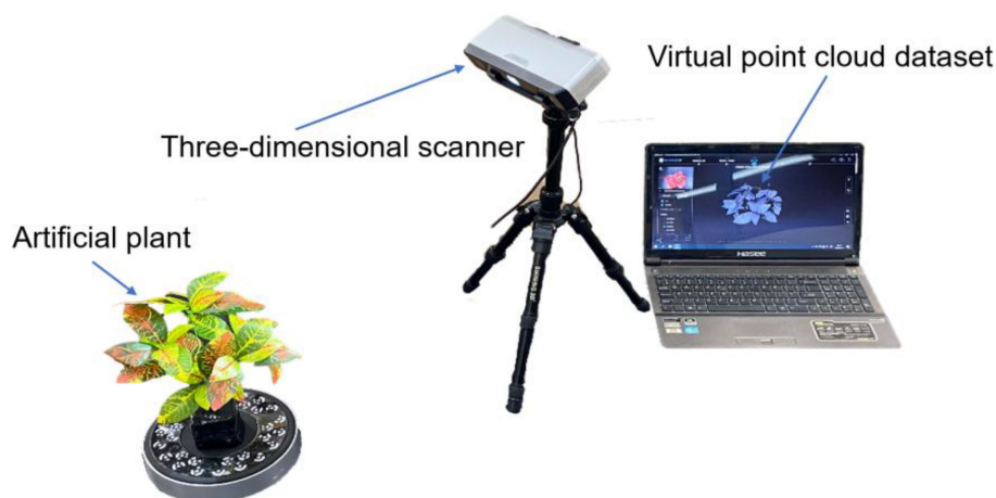
FIGURE 4 Three-dimensional scanner scanning of artificial plant physical model.
