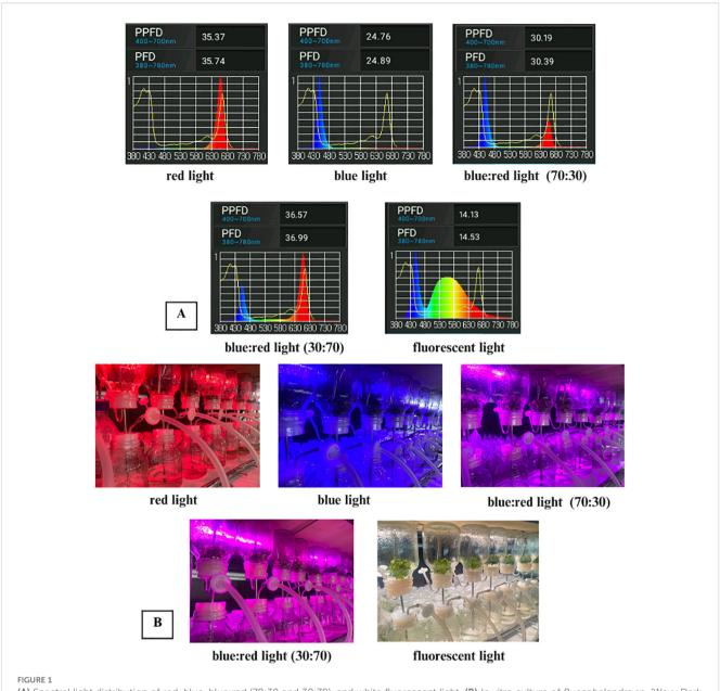
(A) Spectral light distribution of red, blue, blue:red (70:30 and 30:70), and white fluorescent light. (B) In vitro culture of Bucephalandra sp. 'Wavy Dark Green' in a temporary immersion bioreactor system (TIS) under different light quality treatments: red, blue, blue:red (70:30), blue:red (30:70), and white fluorescent light.
