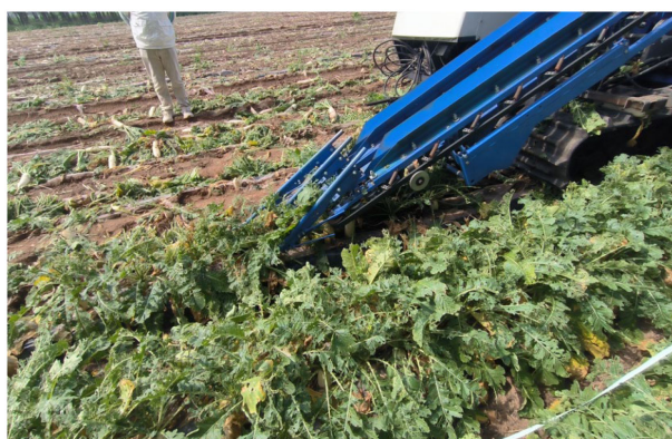
FIGURE 19 Field experiment on the petiole extraction process in radish harvesting.
