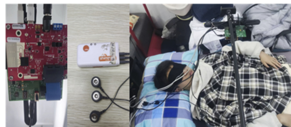
FIGURE 7 Radar sensor, Shimmer ECG sensor and experimental scene.
