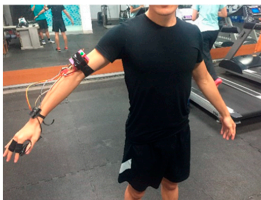
FIGURE 5 A photograph of the WHDD on the human arm. Reproduced from: Lin S-S, Lan C-W, Hsu H-Y, Chen S-T. Data analytics of a wearable device for heat stroke detection. Sensors . 2018; 18(12):4347. Licensed under CC BY 4.0 (Lin et al., 2018).
