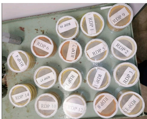
FIGURE 2 The prepared gold tailings soil samples in Marinelli beakers.
