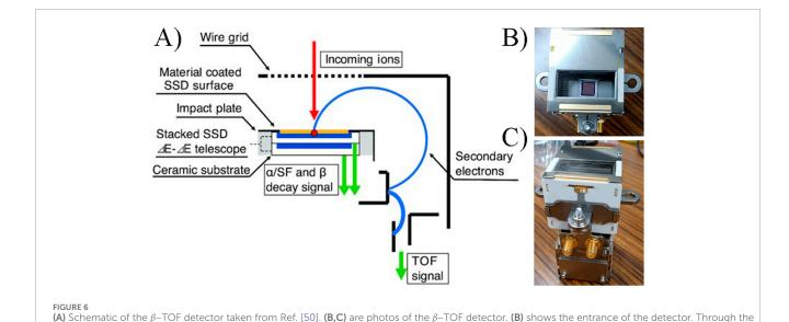
wire grid, the front-side SSD - implanted into the impact plate of the detector - is visible. (C) shows two additional SMA connectors, which were
