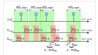
FIGURE 7 Schematic illustration of  $\beta$ - $\beta$  and  $\beta$ -TOF coincidence events. Events detected by the TOF and silicon detectors are represented by blue and red circles, respectively. The green and red filled rectangles indicate the time windows defined by the corresponding TOF and  $\beta$  events for the  $\beta$ -TOF and  $\beta$ - $\beta$  correlated measurements, respectively. Note that the time windows are not drawn to scale for clarity.
