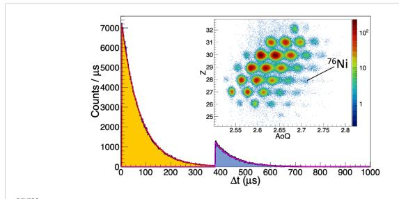
FIGURE 3 Fitted distribution of time intervals between consecutive events measured with the DDAQ system (orange-filled) compared with that obtained using the BigRIPS CAMAC DAQ (blue-filled). The inset presents the associated PID spectrum. The CAMAC DAQ's 337 µs deadtime is clearly visible in the blue-filled curve.
