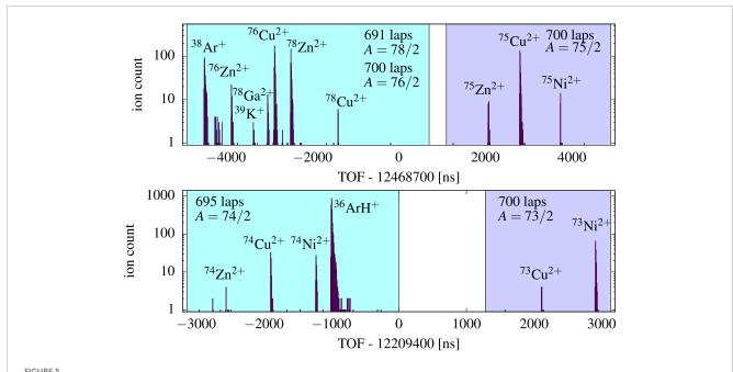
Top: Time-of-flight spectrum for A/q = 75/2, 76/2, 78/2 isobars (radioactive ions in  $2^+$  state), where the IMD has been preset to transmit A/q = 75/2, 76/2, 77/2 (A/q = 77/2 not abundant). Color shades indicate expected regions for different isobar chains. One can see limitations due to the presence of 78Ga/Zn/Cu<sup>2+</sup> ions transmitted along with the other isobar chains without intention (see text). Bottom: Time-of-flight spectrum of A/q = 73/2 and A/q = 74/2 isobars.
