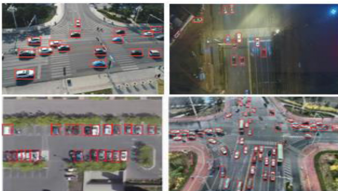
FIGURE 4 RNN based vehicle detection on day and nighttime UAV imagery sample frame with predicted bounding boxes.
