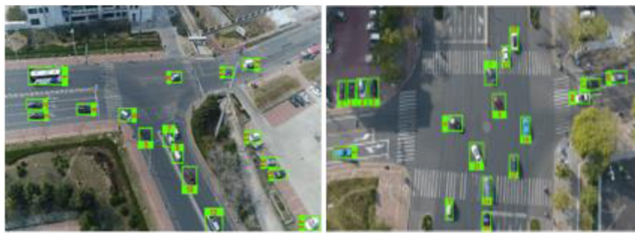
FIGURE 6 Vehicle tracking via DeepSORT algorithm.
