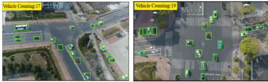
FIGURE 5 Vehicle counting results using the temporal enhancement optical flow (TE-OF) method, illustrating dynamic object motion tracking and accurate frame-wise vehicle enumeration.
