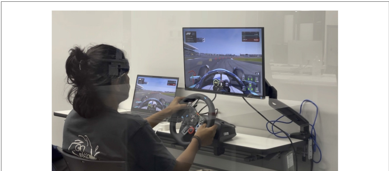
FIGURE 2 Photograph of the experiment scene. A participant equipped with a Muse S wearable EEG headband operates a high-fidelity F1 racing simulator featuring a Logitech G29 force-feedback steering system and pedals on the laser-scanned Silverstone Circuit within a controlled laboratory environment.
