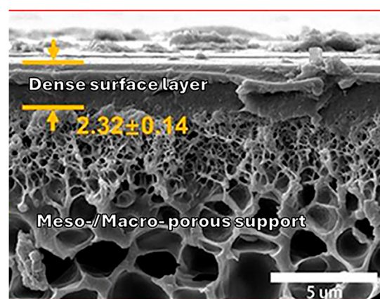
FIGURE 11 Cross-sectional SEM of an asymmetric membrane formed by NIPS of a solution of PSf in a good solvent mixture of dimethylacetamide (DMAc) and tetrahydrofuran exposed to ethanol as a nonsolvent. Adapted from Mei et al. (2020).
